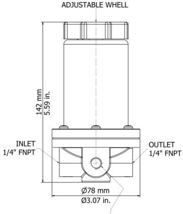
1/8" FNPT PLUG OR PRESSURE GAUGE FIT
