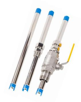
LECOL B7X series pH sensor are installed directly into pressurized processes through a 1-1/4" ball valve assembly. The sensor design has a flared safety tip which prevents accidental ejection during removal of the sensor from the process.
